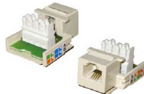
T-K024 Cat.3 RJ45 Keystone Jack A: 110IDC B: Screw Type
